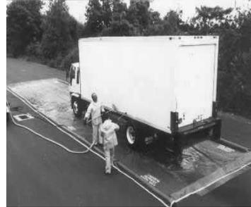
**Vacuums/Pumps** – Devices such as wet/dry vacuums, sump pumps, and vacuum pumps may be used to collect wastewater after pressure washing. Vacuum devices typically have an extension (vacuum boom) which allows the wastewater to be collected efficiently. In addition, many vacuum devices are designed with a second hose (e.g. garden hose) that can run from the pump to the sanitary sewer or a truck/trailer mounted holding tank, depending on disposal method.
